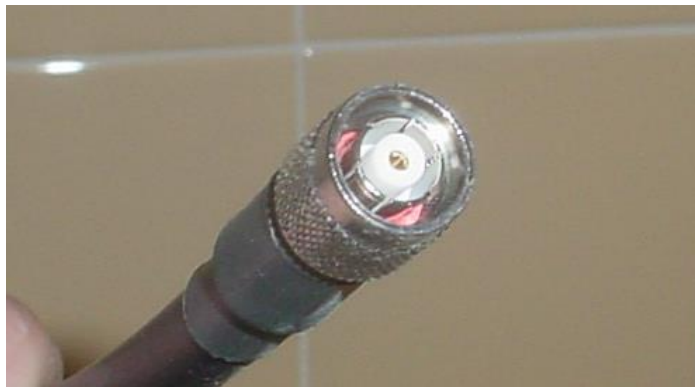
FIGURE 3: The RP-TNC Plug connector end of the 400-series cable will terminate at the closest wireless data outlet as indicated on the floor plan. No more than 1-1/2' of the 400-Series Cable will be exposed at the wireless data outlet location. The cable will be installed above the freezer, fastened down at 12" intervals and any excess cable will be coiled above the entry point into the freezer. The 400-series cable will not be installed in conduit, except the 12" conduit length through the cooler ceiling. A moisture-impervious seal is required inside
