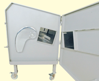
Model 109PC & 109PCM Left door open showing a Sickle-type smooth Blade and the Surplus Catch Tray. The Stainless Steel Catch Tray allows the further use of the slicer's product's surplus pieces. Use pieces for stir fry, fajitas, and for further processing like ground meat. This advantage qualifies this machine to have a virtually zero waste operation.
