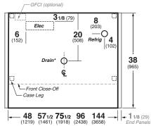
\*Drain position is for 48" length only, refer to Cadblock drawings for other lengths
